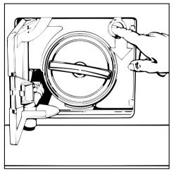
Pull the ring of the door mechanism downwards, the door will open.
